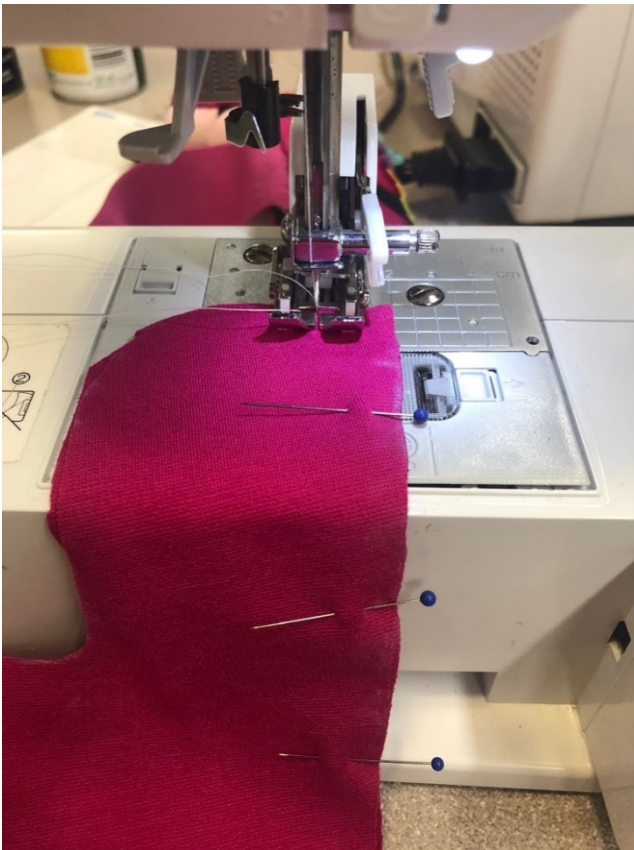
Figure 6. Ponte De Roma seam allowance reduced.
