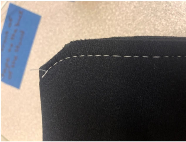
Figure 7. Neoprene piece with seam allowance trimmed.
