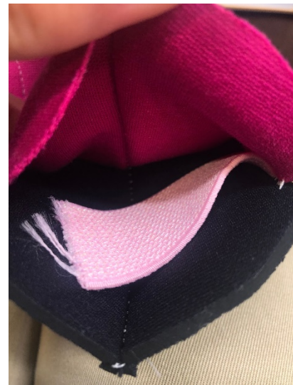
Figure 9. Elastic sandwiched between fabric pieces.
